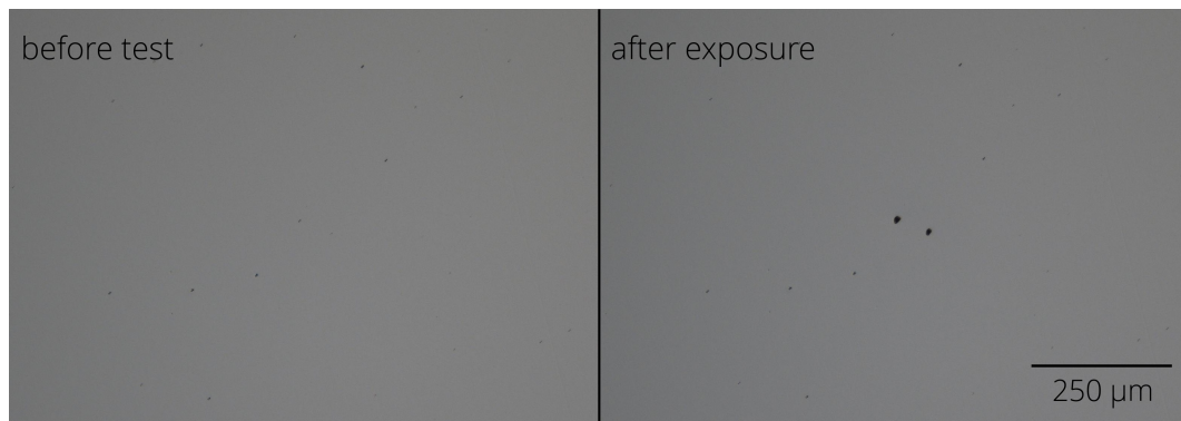
Figure 5. Typical damage morphology: fluence 1.65 \text{ J/cm}^2 , damage after 110 pulse(s).
